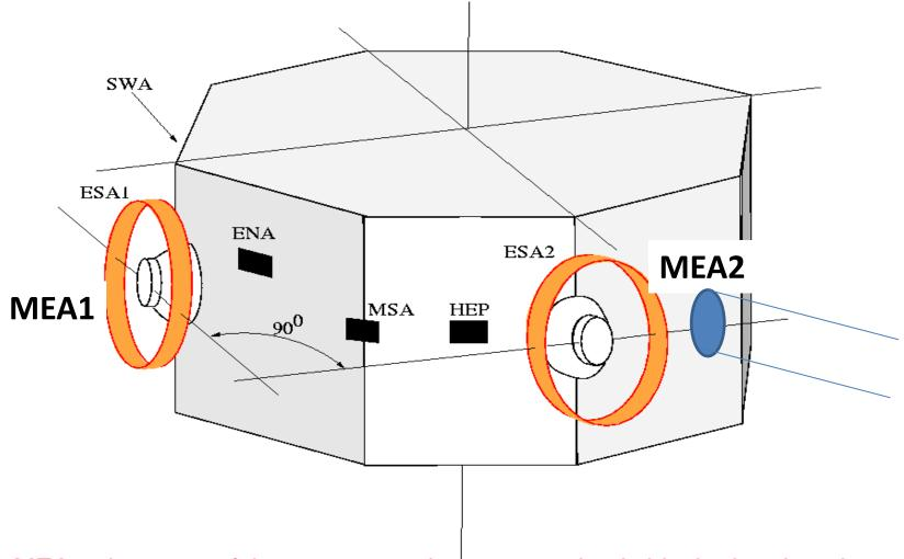
MEA-2: because of the mast 2 anodes are completely blocked and 2 others are partially obscured
