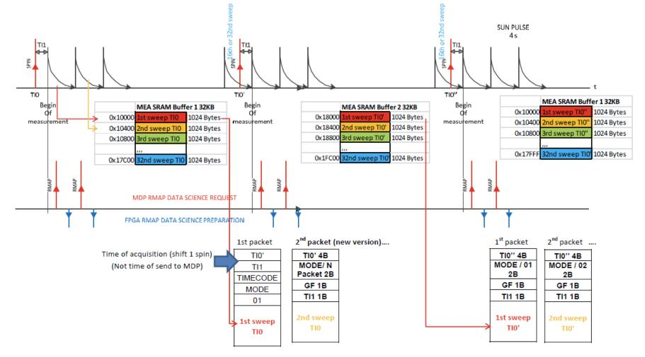
Time of acquisition (shift 1 spin) = TIO' + TI1 + (n° packet – 1) x Tspin / 32 or (Tspin /16)
