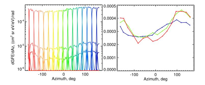
Left: Azimuth response of the 16 anodes for 3 values of the geometrical factor Right: GF in linear scale versus azimuth. The blue, green and red curve respectively correspond to Utop/Uan=0.85, 0.3 and 0.25. GF values are normalized to the maximal GF.
